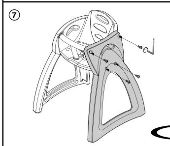
Stand chair upright and insert x4 Allen Bolts Tighten securely using Allen Key provided
