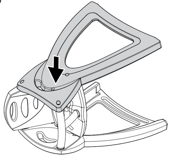
Push Side Support Leg firmly down to ensure a good fit
