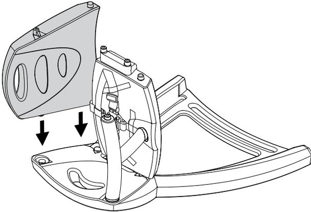
Insert Back Support. Push firmly to ensure a good fit
