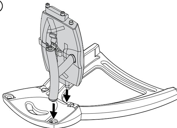
Lay x1 Side Support Leg on a flat surface
