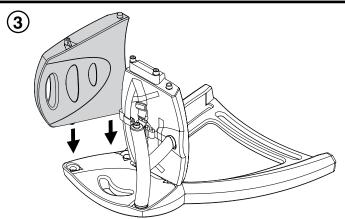
Insert Back Support. Push firmly to ensure a good fit Note: Ensure Safety Strap is still taped to Seat Pad
