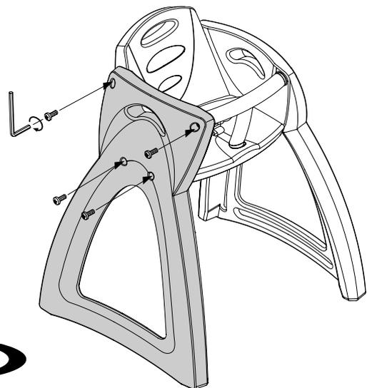
Rotate chair and insert other x4 Allen Bolts and tighten securely using Allen Key. Remove Tape from Strap - Your chair is ready to use.
