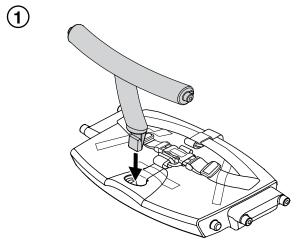
Insert 'T' Bar into Seat Note: Leave Safety Strap Taped to Seat
