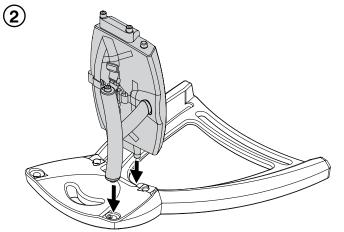
Lay x1 Side Support Leg on a flat surface Insert 'T' Bar & Seat into Side Support Leg Push firmly to ensure a good fit
