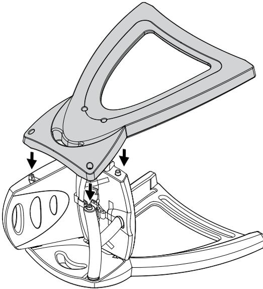
Locate other x1 Side Support Leg onto rest of already assembled components
