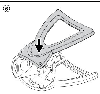
Push Side Support Leg firmly down to ensure a good fit
