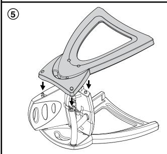
Locate other x1 Side Support Leg onto rest of already assembled components
