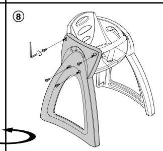
Rotate chair and insert other x4 Allen Bolts and tighten securely using Allen Key. Remove Tape from Strap - Your chair is ready to use.
