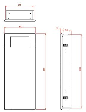
Height: 836mm Width: 342mm Depth: 120mm Weight: 9Kg Capacity: 18 Litres
