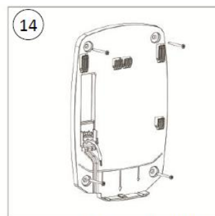
Screw the Plug-in base to the wall(x4)
